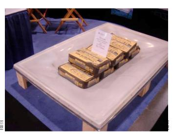
Both products pictured can support a 200-pound weight with obvious strength differences. However, all plastics age when exposed to of UV from the sun over time. The question is can a plastic skylight of any kind withstand the weight of a falling worker or object when new or when exposed to 10 to 20 years of UV from the sun?
